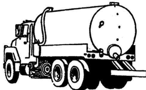
*A typical haulage truck used to pump septage (raw sewage) from septic tanks and holding tanks and dispose the contents directly to the surface of land or at waste treatment facilities.*
